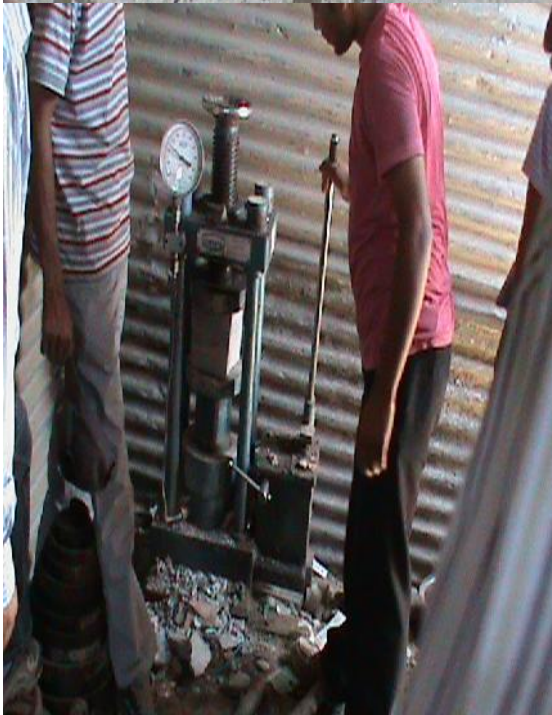
Cement concrete cube taken at site, machine testing the strength of old cubes
