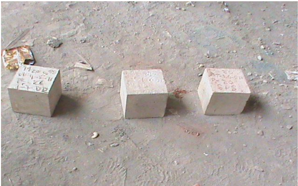
Various cement concrete cubes taken for quality testing during the execution of the project
